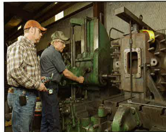
■ (Left) Compressor Elements can reline cylinders up to 26 in. (66 cm) diameter. Compressor Elements has just added this new "State-of-the-Art" Mazak QTN-450M to its list of CNC machines (right).
