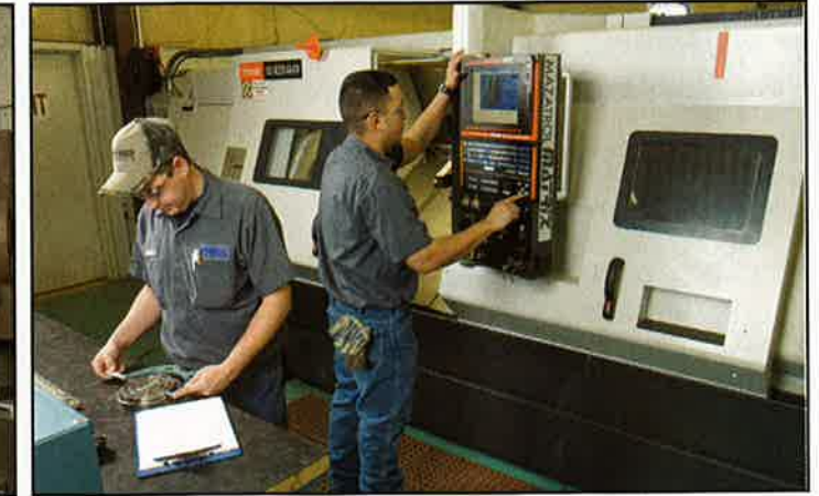
■ (Left) Compressor Elements can reline cylinders up to 26 in. (66 cm) diameter. Compressor Elements has just added this new "State-of-the-Art" Mazak QTN-450M to its list of CNC machines (right).
